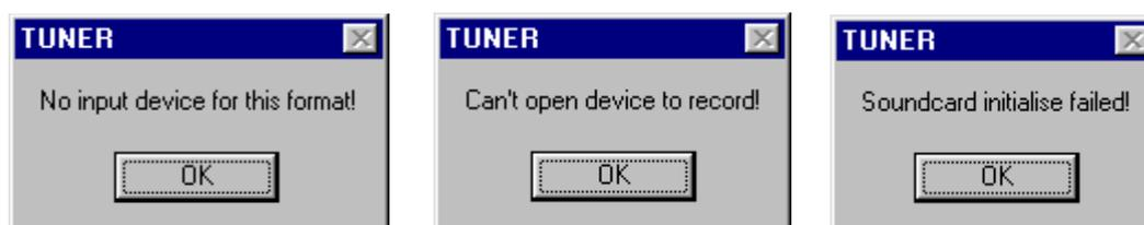
there is some problem with Tuner accessing the soundcard on your PC. Make sure that a soundcard is fitted, it is recognised by Windows (e.g. you can play sounds through it), it supports the sound-file format used by Tuner, and that no other program is accessing it at the same time as Tuner.
